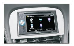
Connect all required circuit points to the head unit and and push it into the metal frame until it snaps in. Place the trim frame.
