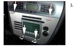
Insert 4 radio release keys into slots on the top and bottom of the radio (see arrows)
