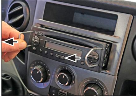
1. Remove OEM head unit with radio release keys
