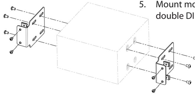
5. Mount mounting brackets to double DIN head unit
