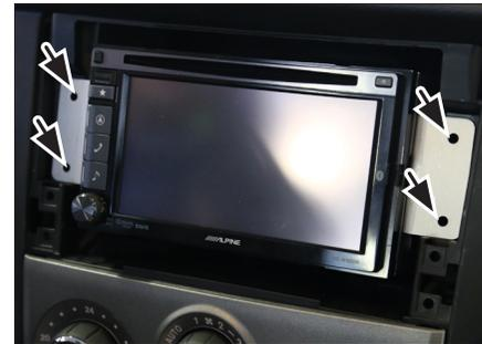
7. Fix double DIN head unit with 4 screws (see arrows)
