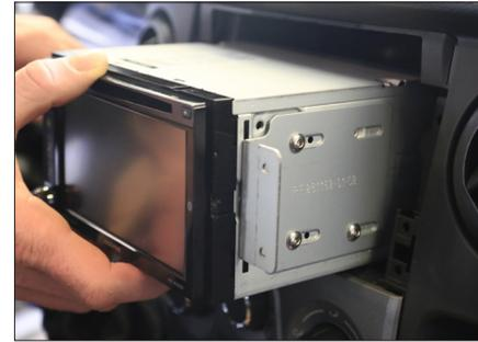
6. Connect all required circuit points. Push double DIN head unit into dashboard
