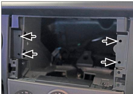
4. Put four speed nuts in the openings of dash board
