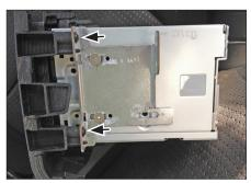
4. Attach metal mounting frames to Double-DIN head unit
