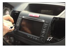
Remove screws of OEM head unit (see arrows)
