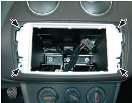
3. Fix the new mounting frame with the 4 original screws.
