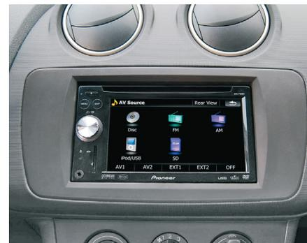
4. Connect all required circuit points and push the double DIN head unit until it snaps in.
