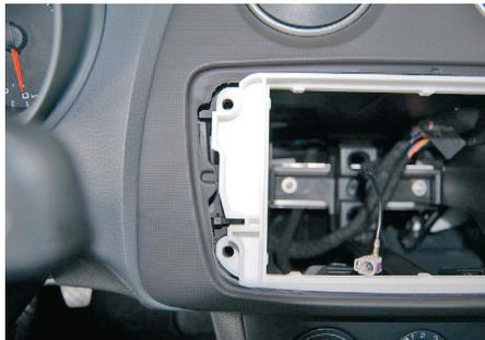
2. Place the new mounting frame (see photo) into the dashboard.
