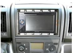
5. Connect all required circuit points and push the double DIN head unit until it snaps in.
