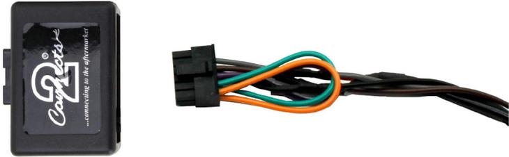
3. Connect the opposite end of head unit patch lead to the head unit steering wheel control input on the back of the aftermarket head unit. This may be a 3.5mm jack plug or a wire input depending upon the head unit brand being fitted.
