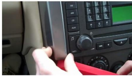
Using appropriate tool un-clip, the surround panel as shown.
