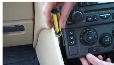
Remove the screws from either side of the air con unit.
