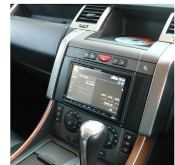
Fit the head unit into the cage, then fit the replacement panel.
