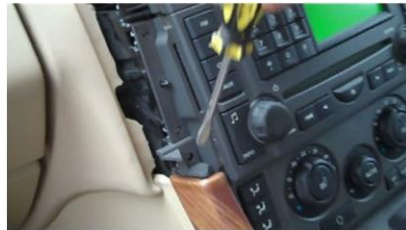
Unscrew the screws around the head unit.
