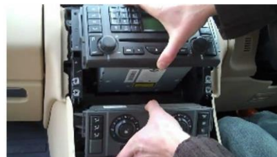
Unclip the head unit and remove.
