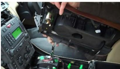
Taking care unplug switches and remove panel as shown.
