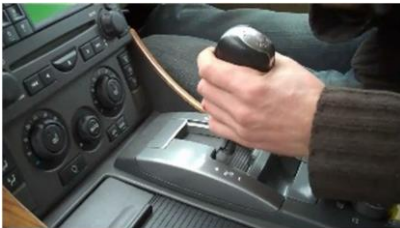
Pull the gear stick up and remove.
