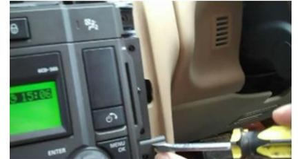
Unscrew the screws around the head unit.
