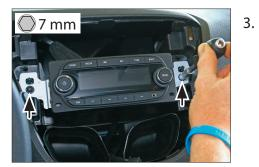
Remove 2 screws of OEM head unit (see arrows). Put the OEM screws aside because they will be used later
