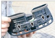
7. Place air vents onto new 2-DIN facia plate
