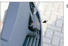
8 . Place hazard light switch onto new 2-DIN facia plate
