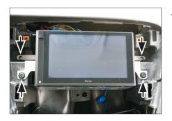
10. Connect all cables Place 2-DIN head unit onto dash board
