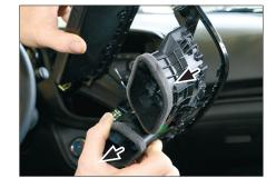
6. Unclip and remove air vents from OEM panel
