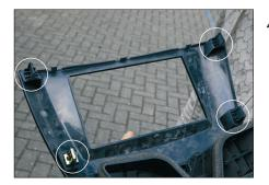
4. Remove 4 clamps from OEM panel Place4 clamps onto new facia plate
